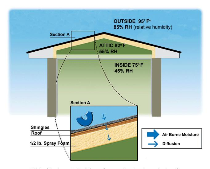
Think of the "unvented attic" as a foam cooler placed over the top of your house. It stops over 90% of the sun's radiation and all the air infiltration.
